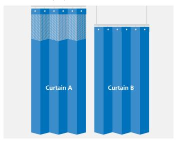
**Curtain A:** Track fixed to ceiling may require curtains with 50cm mesh top section to allow for sprinkler system. These curtains have a 2.3m drop.
